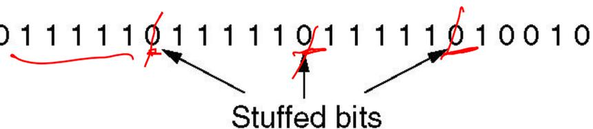
Diagram showing bit stuffing with arrows pointing to stuffed 0s.
